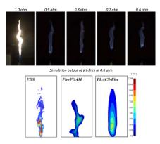
Accidental jet fires occurring in industrial facilities can involve severe consequences as they can trigger domino effect. The assessment of the flame-geometry descriptors of the jet can contribute to prevent flame impingement on plant equipment, hence reducing inventory loss
