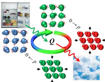
They also identified the reversible range where barocaloric effects can be implemented in a device working upon cyclic application and removal of pressure. The study should inspire the development of future environmentally-friendly solid-state barocaloric cooling devices.
